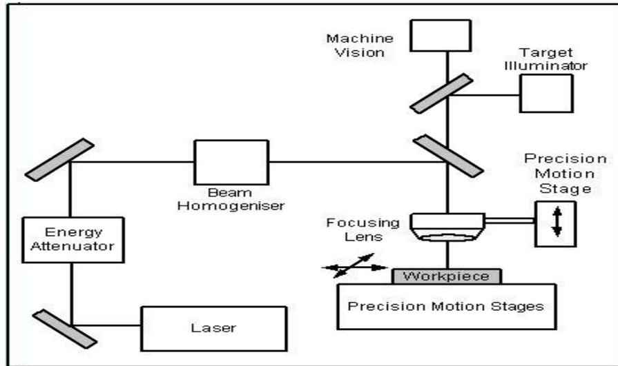
**Conceptual Solid Model of Laser Micromachining Setup**
