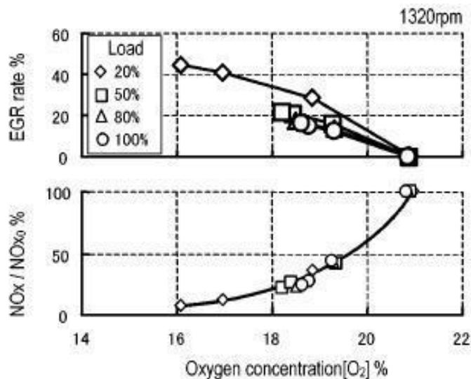
**Fig 2 Relationship between oxygen concentration and NOx reduction**
