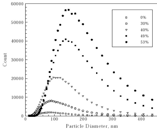
**Fig 10. Time-averaged size distributions as measured by the SMPS.**
