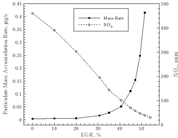
**Fig 9. Relation of PM Accumulation Rate and NOx emission with EGR.**
