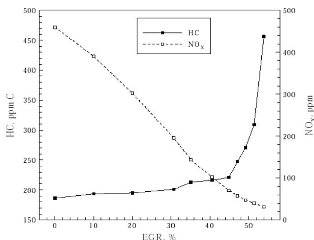
**Fig 8. Trade-off between HC and NO<sub>x</sub> concentration as a function of EGR Level**
