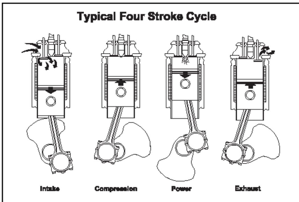
**Fig 1. Working of four stroke engine.**
