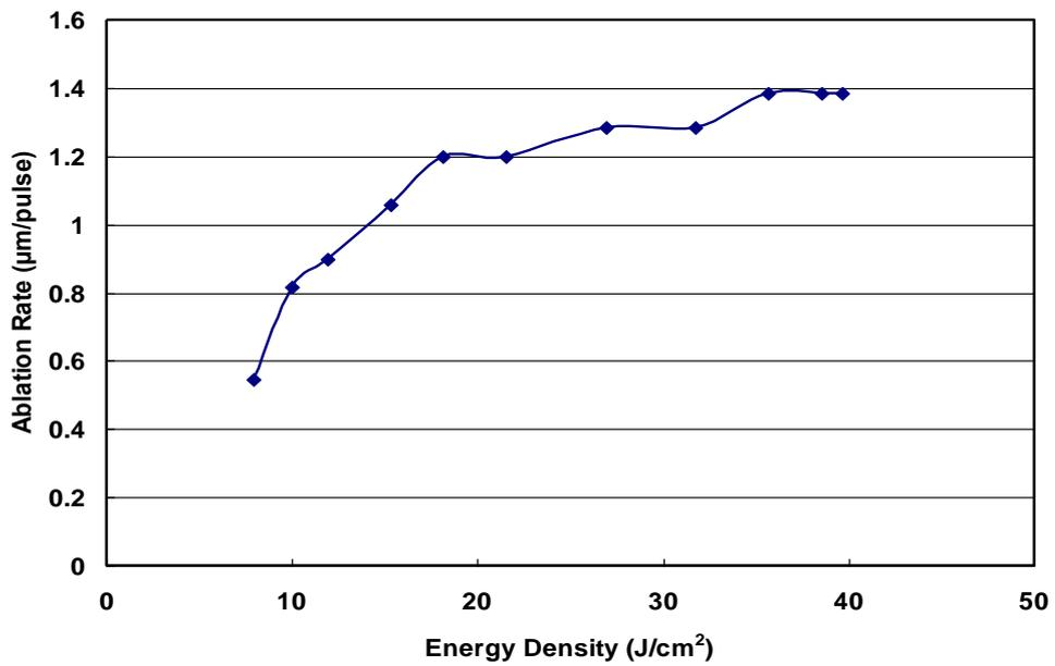
**Optimization of Pulse Energy Required to Drill Holes**
