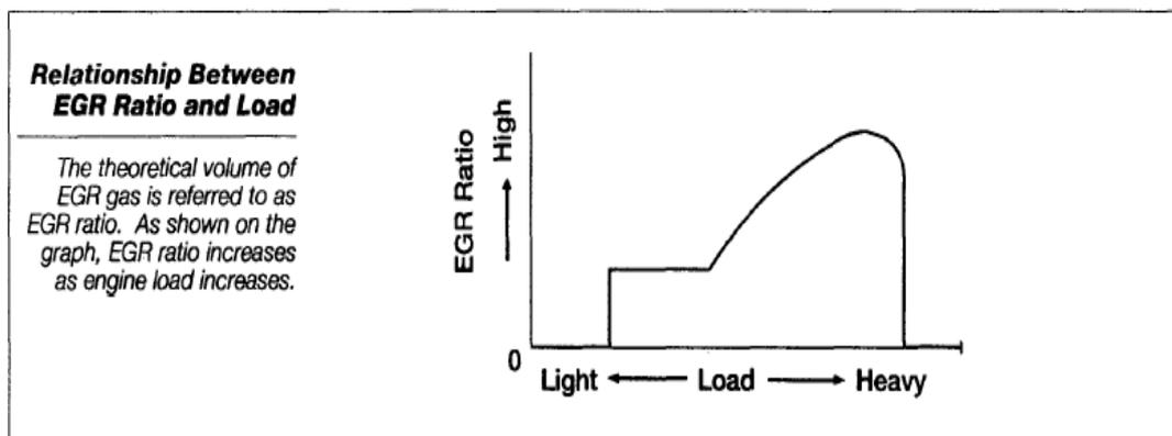
**Fig 7. Relationship between EGR Ratio and Load**
