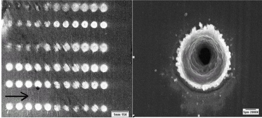
Holes drilled in 25µm thick brass foil
