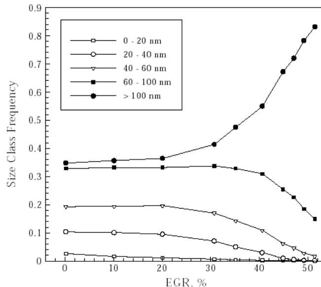
**Fig 11. Frequency of occurrence of particle size classes as a function of EGR.**
