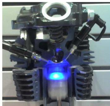
**Fig.1. DTSI Engine (Courtesy: Bajaj Pulsar Bike)**
